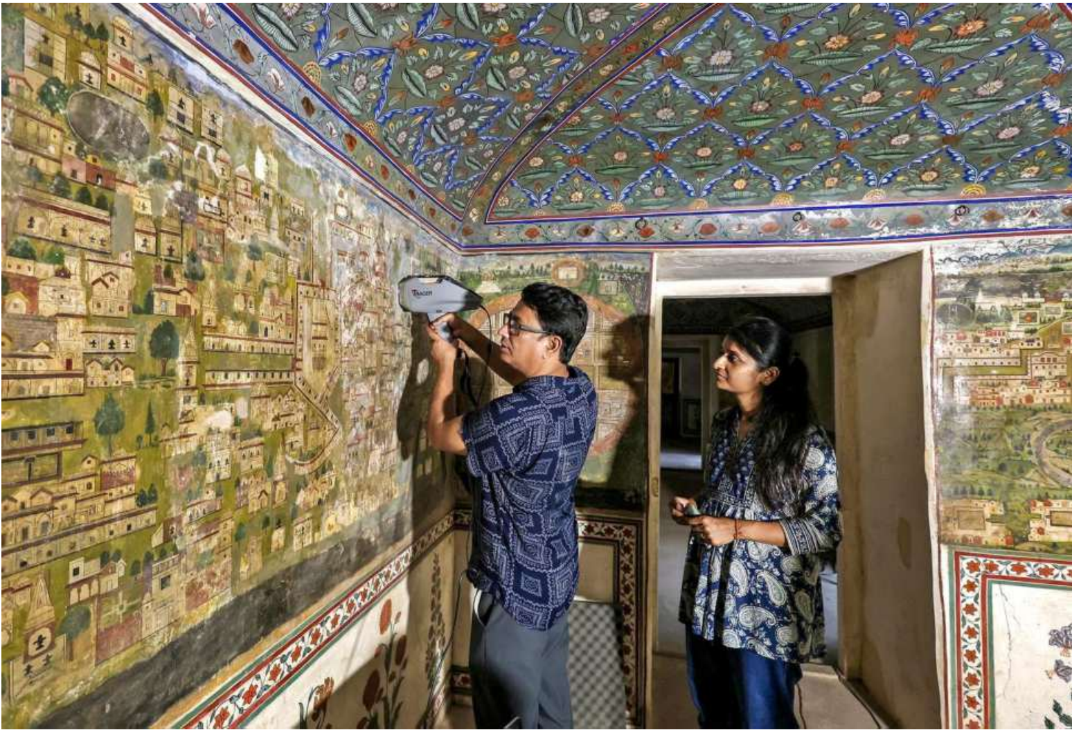
Experts from the Indira Gandhi National Centre for the Arts use a portable X-ray fluorescence analyser to examine the pigments, material composition and condition of centuries-old frescoes during their scientific documentation and conservation at Amer Fort, in Jaipur, Rajasthan, on July 24. PTI
