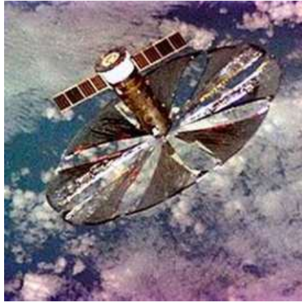
Eärendil-1 won’t be the first mirror in orbit. Shown here is Znamya-2, which Russia deployed as part of a series of orbital space mirror experiments in the 1990s. RSC ENERGIA
