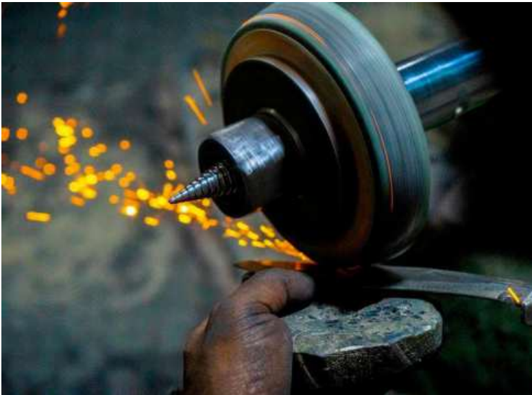
Razor sharp: A worker shapes and sharpens the khukuri on a machine during the finishing process.
