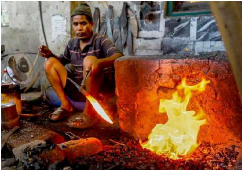
Generational craft: A craftsman heating a khukuri knife in a furnace before shaping it by hand in Patan, Nepal. The skills have been passed down through generations.
