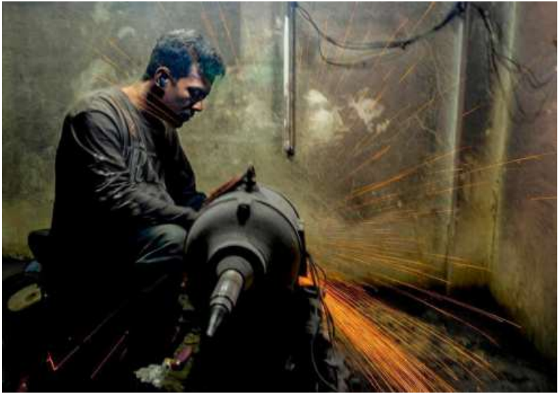
Final touches: The knife is sharpened on a machine during the finishing process in a traditional workshop.
