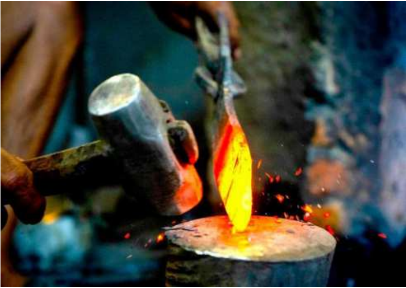
Precise detailing: A blacksmith shapes a red-hot khukuri blade with a hammer during the traditional forging process at a workshop.
